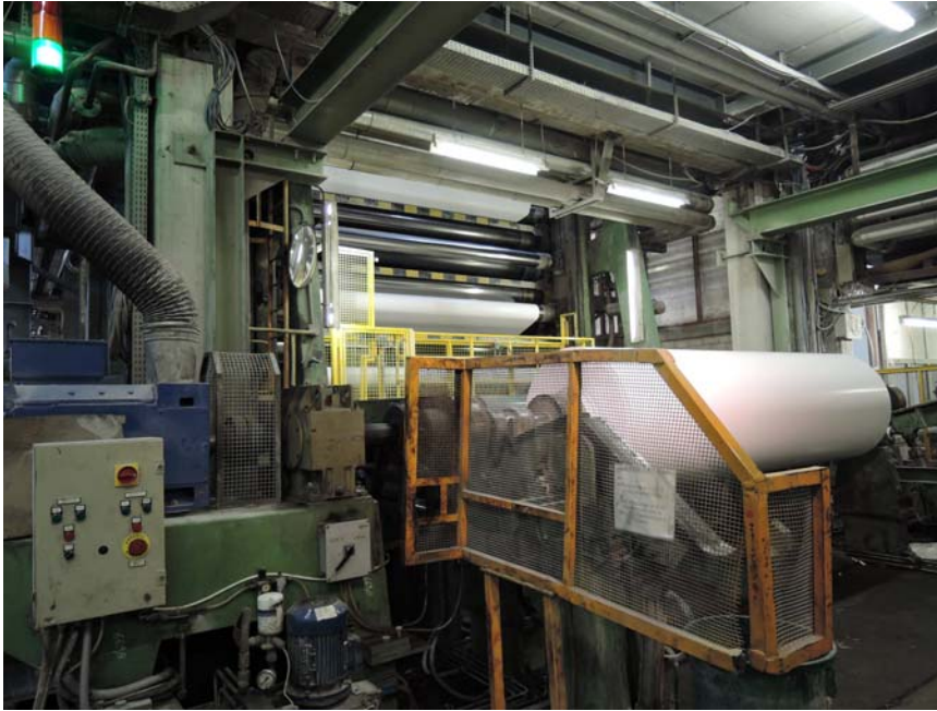
KLEINEFEGERS SUPERCALANDER reconstruction together with the BRUDERHAUS Drive made on site.
