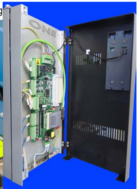
One board fits all our Drives, DC-AC-BRUSHLESS-CHOPPER and REEBORN (the system who saves the original Drives, all brands included) of the “INTELLIFLEX PLATROFM ONE DRIVES”
