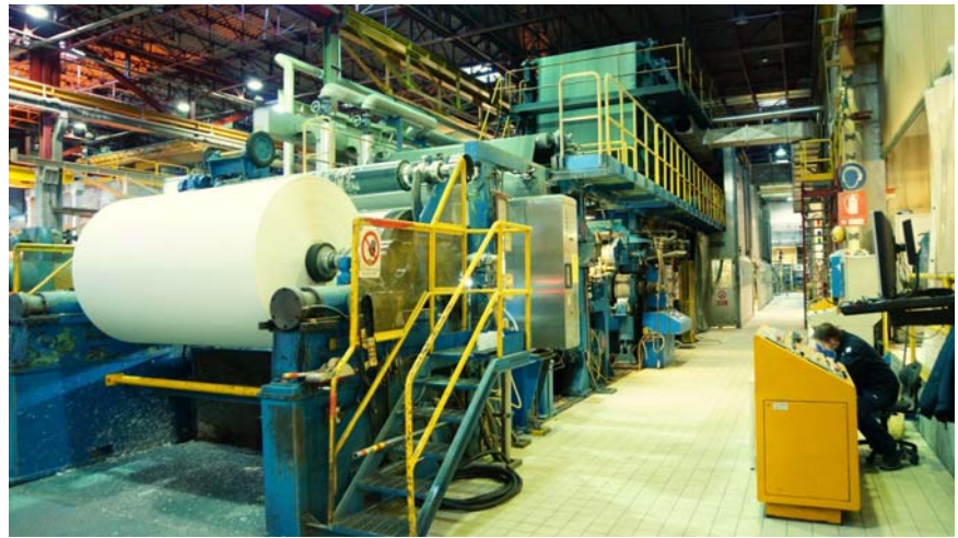
MC3 – POPE Zone – Rebuild on 2016 in two steps by “ONE PLATFORM”, the flexible and powerful sectional drive system who never get old.
