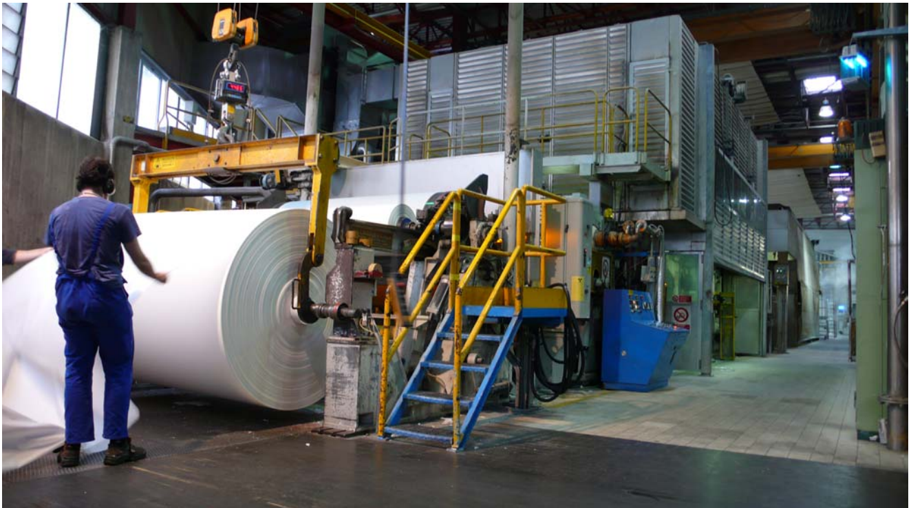
Machine 1 - POPE Zone – Rebuild on 2013 in two steps, “ONE Drive” PLATFORM SAEL
