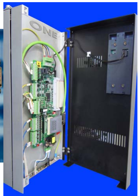
The only one regulation card - same Hw for all our drives. DC-AC- BRUSHLESS-CHOPPER and REBORN ( system that reused all the DC drives of any model) of series "PLATFORM ONE DRIVES"
