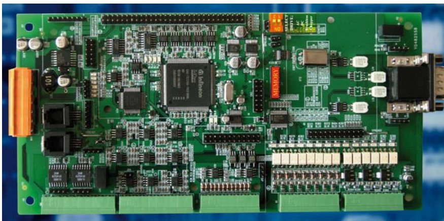
The only one regulation card - same Hw for all our drives. DC-AC- BRUSHLESS-CHOPPER and REBORN ( system that reused all the DC drives of any model) of series "PLATFORM ONE DRIVES"
