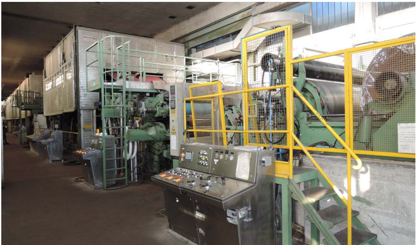
Pope, Calander and Driers of SACI-PM3 equipped with inverter liquid cooled.
