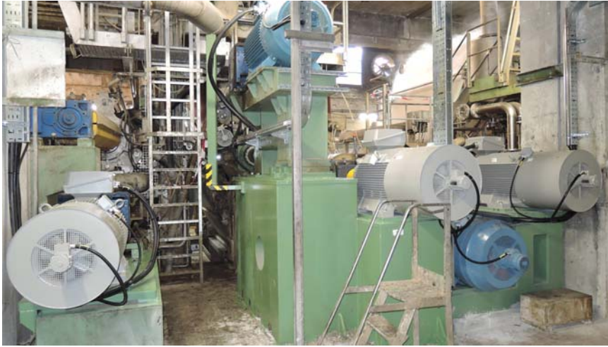
All the motors AC we included in the scope of supply, cartiera PM3- Press
