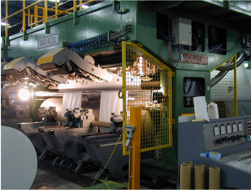
Rebuilding of Teleset, Telebok ed LDS in a VariRoll winder
