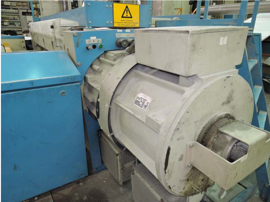
Blade Drive Unit – One of the two Brushless systems, Sarego, Burgo Group
