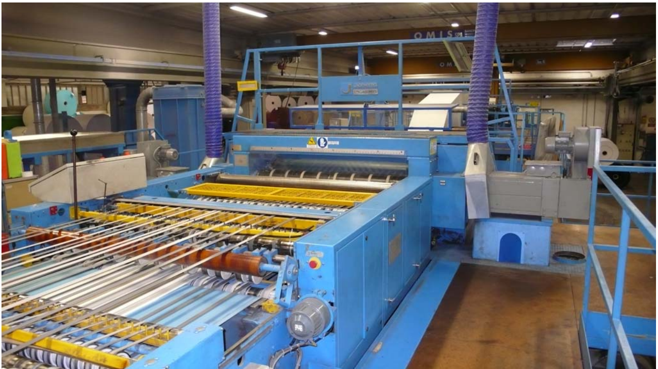
The Jagemberg sheeter subject of the SAEL revamping: Total atomization and DC motors replacements with AC low inertia motors - SAEL "PLATFORM ONE DRIVE".
