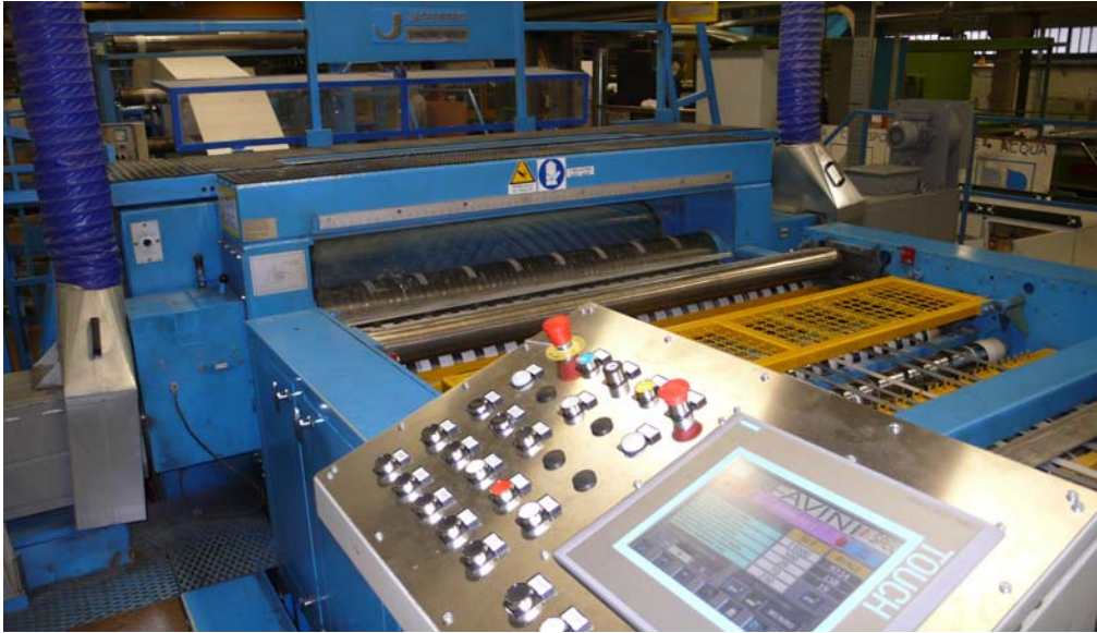
The main control Desk drive rebuilt and simplified to a more ergonomic and modern management. The control Desk possesses a touch screen video-keyboard.
