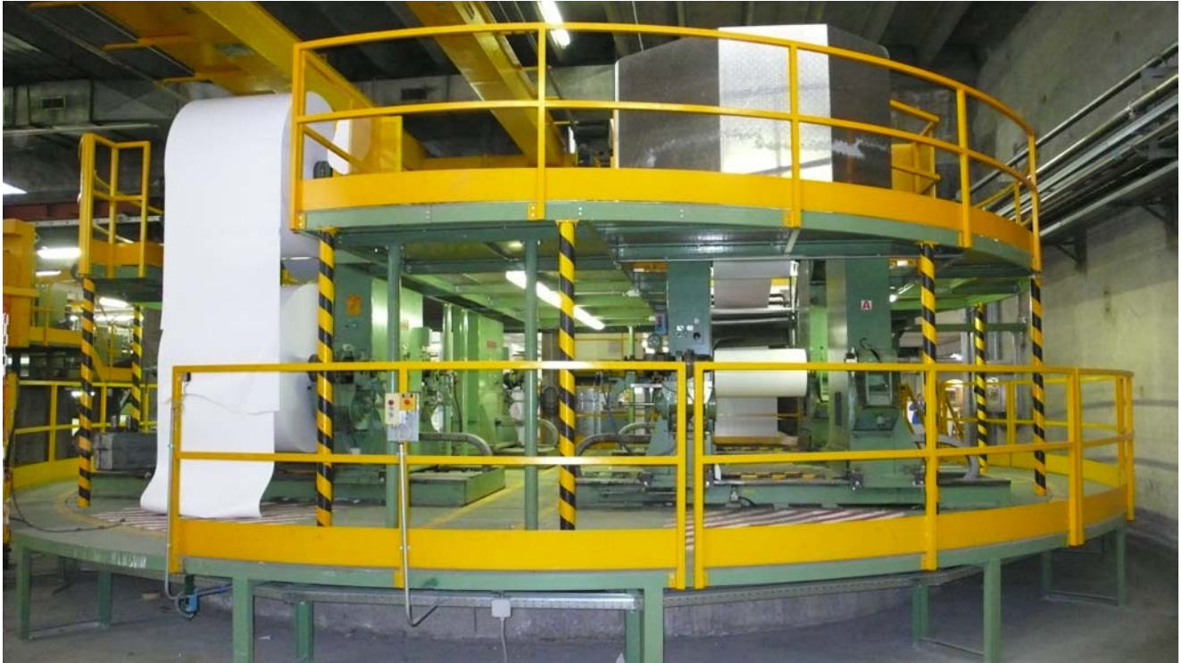
turning reel load device installing degressive braking
