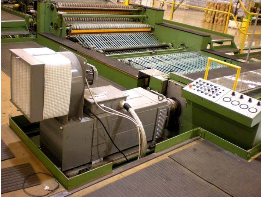
Above: New knife AC motor after rebuild
