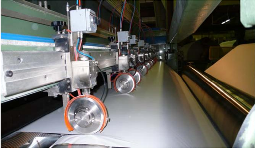
Mantovaa papermill, winder machine knives selection
