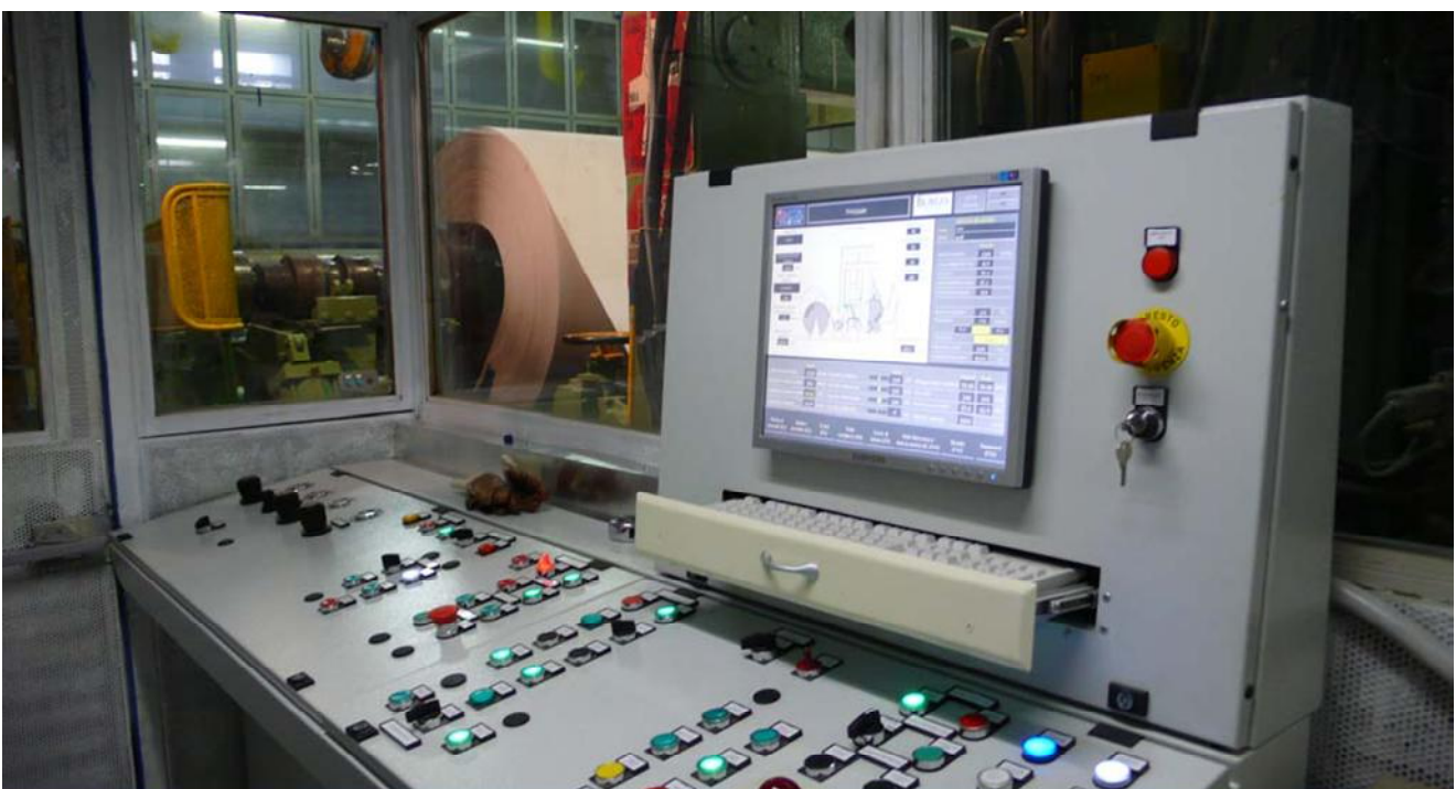
Control pulpit of 7 meters use format winder machine ; run speed 1800m/min
