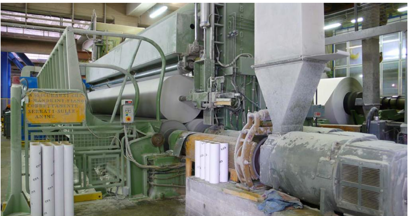
Beloit winding machine carrying drums, Mantua paper machine
