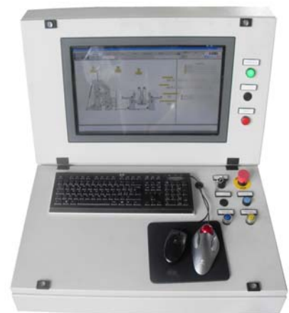
Control Desk of winder with our innovative DCS “WINDER SAEL”
