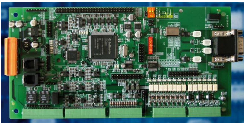
The unique regulation board for all our drives "PLATFORM ONE DRIVES": DC-AC-BRUSHLESS-CHOPPER and REEBORN (the smart device applicable to every drive and brand, in order to replace old drives)
