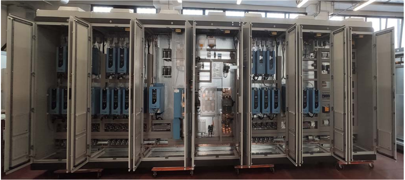
DOUBLE END INVERTERS MOUNTING, FRONT VIEW
