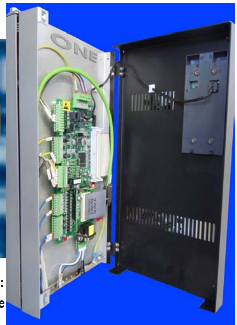
The unique regulation board for all our drives "PLATFORM ONE DRIVES": DC-AC-BRUSHLESS-CHOPPER and REEBORN (the smart device applicable to every drive and brand, in order to replace old drives)
