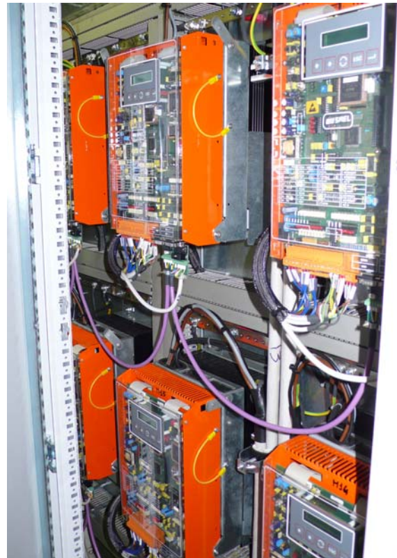
Some of the inverters forming the sectional control of a machine 1
