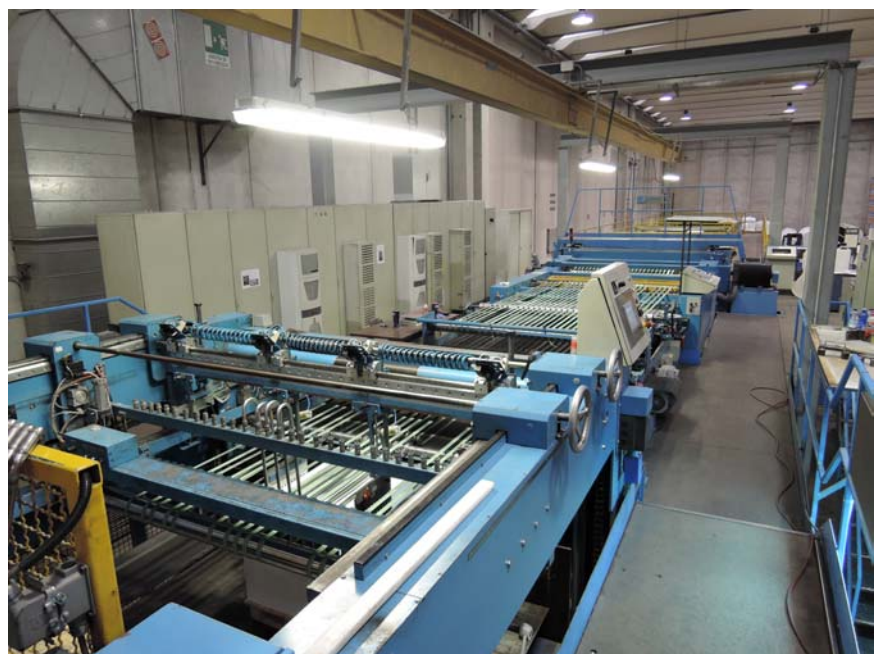
Reconditioned SINCHRO 350-2150 DD2 JAGEMBERG Sheeter at Papiergarda
