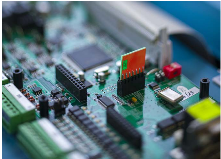
The removable memory mounted into every Board, allowing quick replacements, in case of faults, without settings.
