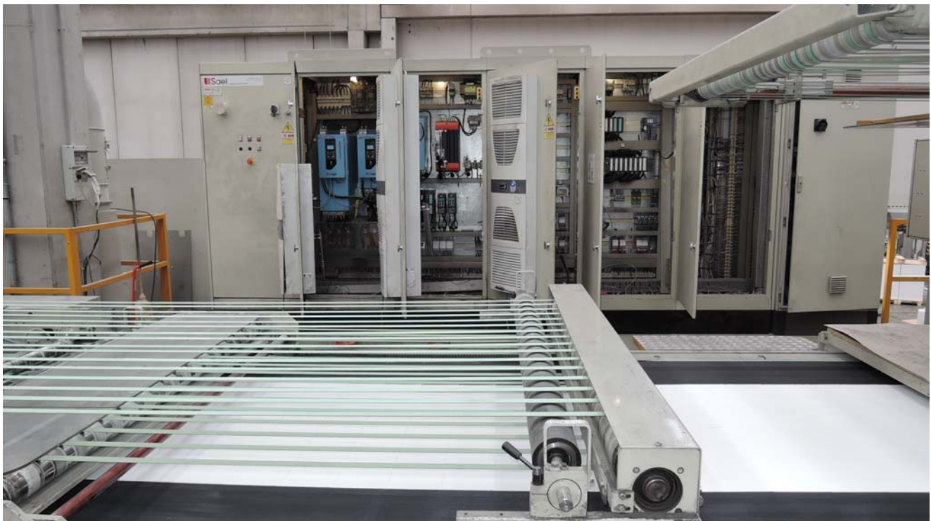
Papier Garda: PIZZOLATO Sheeter completely revamped. Electrical equipments. Global overview.
